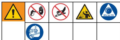
This equipment stays pressurized until pressure is manually relieved. To help prevent serious injury from pressurized fluid, such as skin injection, splashed fluid and moving parts, follow the **Pressure Relief Procedure** whenever sprayer is stopped and before sprayer is cleaned or checked, and before equipment is serviced.
